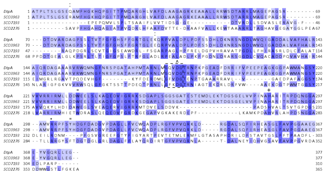
Figure 4.28: Sequence alignment of DtpA from S. lividans with SCO3963, SCO7193 and SCO2276 from S. coelicolor . Clustal Omega sequence alignment with completely and partially conserved residues coloured in dark to light blue, respectively. Symbols identify the position of important haem pocket residues, with the * showing the position of Arg 369 , the ^ the position of Asp 251 and + the position of His 353 (DtpA numbering). The conserved DyP motif GXXDG is shown by a dashed box. The conserved Trp residue with possible importance in LRET is shown by the “ symbol (Trp 301 in DtpA) and the Tyr residue (Tyr 374 in DtpA) also possible to play a role in LRET is shown by a “ symbol. The changes in amino acids between DtpA and SCO3963 are shown by the : symbol. The Tat signal sequences for DtpA and EfeB are not included in the alignment.
